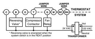
Figure 7. Typical wiring diagram for heat pump with reversing valve energized in HEAT with common connection (required)
